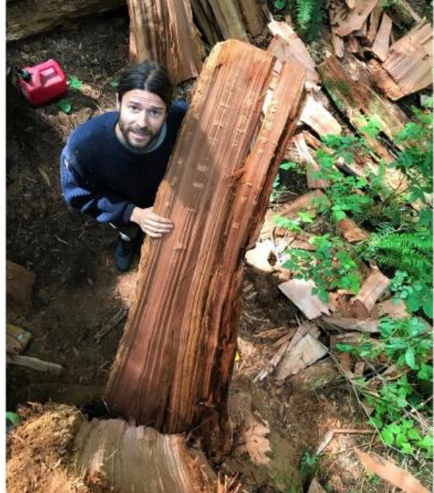
Splitting Western Red Cedar from an old growth stump using an old tool called a fro.
