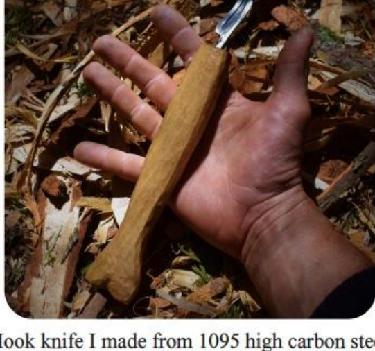
Hook knife I made from 1095 high carbon steel
